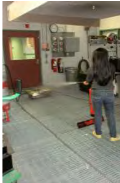
Figure 14: Participant continuously deploys agent on propane fire, thereby preventing re-ignition
